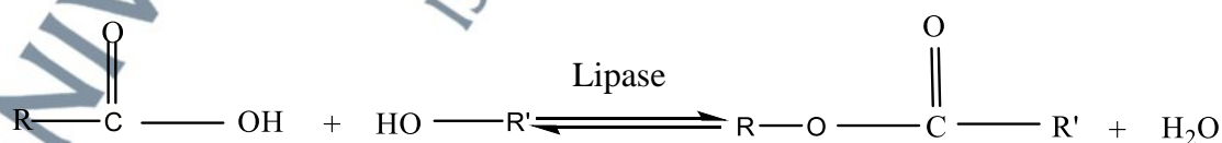
Scheme 2.5: Esterification Reaction of Fatty Acid and Alcohol to Produce Ester
