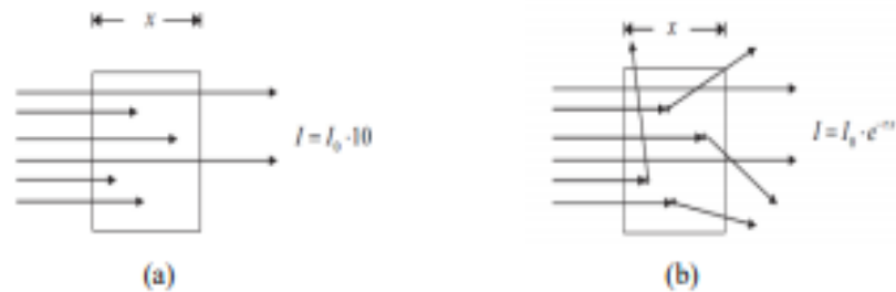
Fig. 1. Transmitted light disturbed by either (a) absorbance (b) scattering [2].
