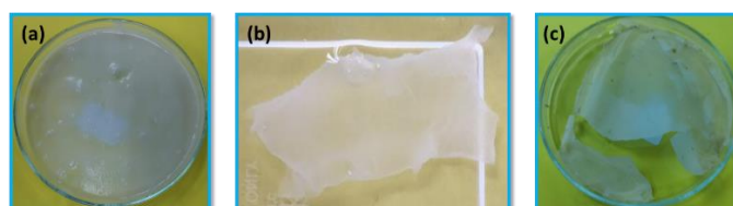
Figure 1. (a) wet EFB cellulose (b) regenerated cellulose/glycerol membrane and (c) regenerated cellulose/glycerol bioplastic
