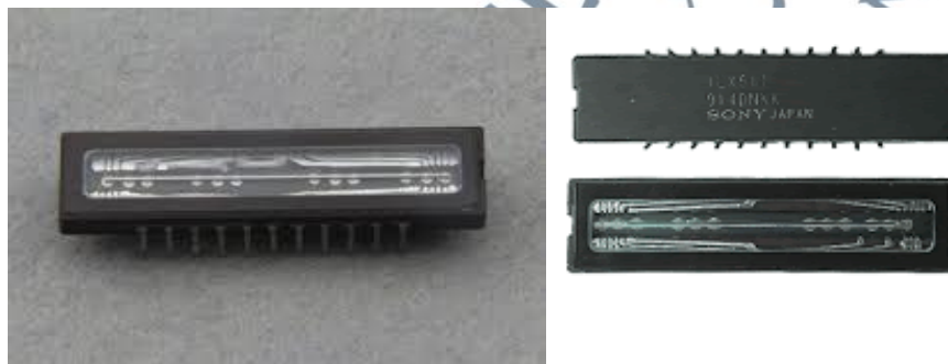
Figure 2.35 CCD ILX551A (Left) and CCD ILX511 (Right).
