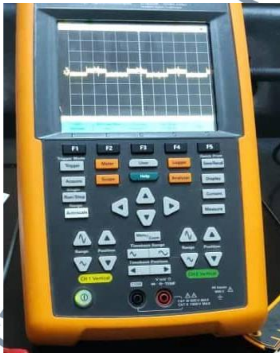
Figure 3.17 Agilent U1620A Oscilloscope Used to Produce the Digital Signal from the CCD Linear Sensor System.
