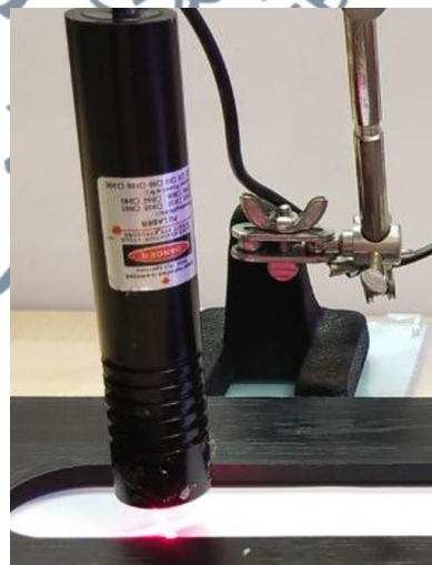
Figure 3.21 Red Laser Diode with 650nm Wavelength.
