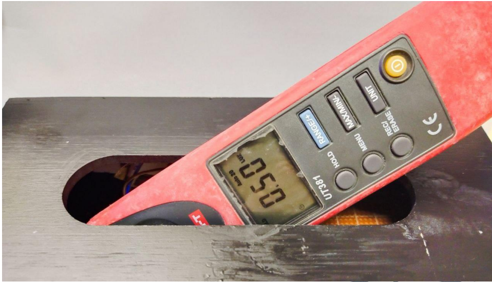
Figure 3.13 A Luxmeter Showing the Light Intensity Inside the Black Opaque Box.
