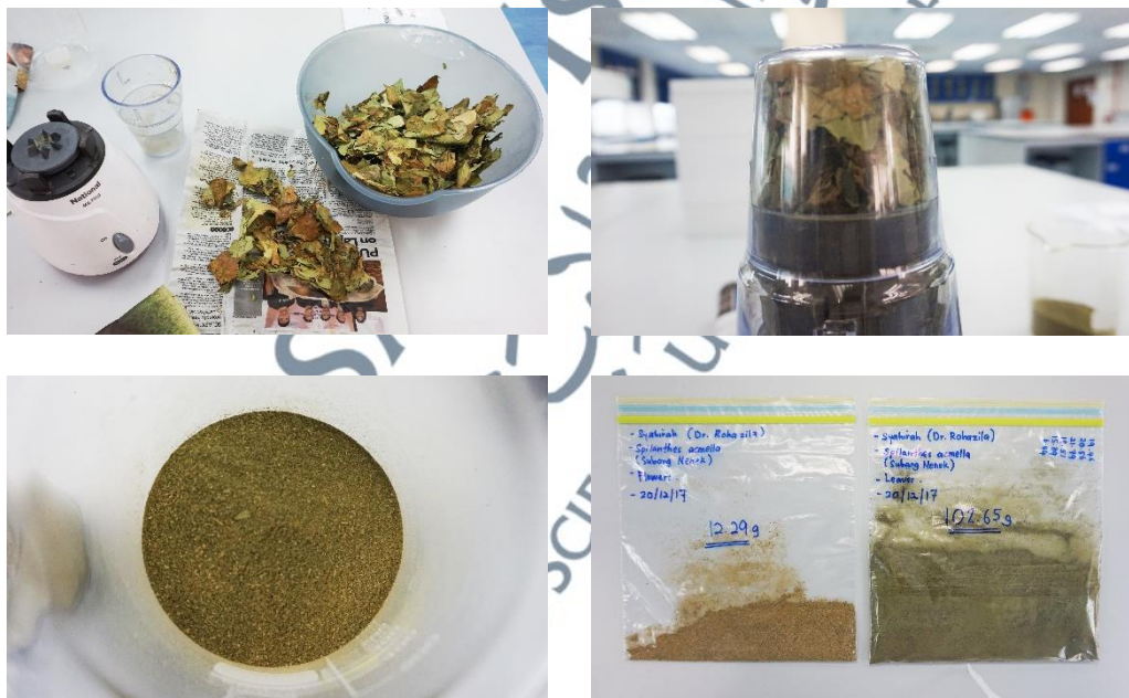
Figure 3.1 (B): The Process of Forming A. paniculata Powder Using a Grinder
