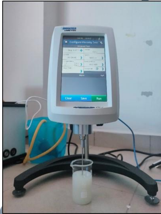
Figure 3.1: Viscosity Measurement of 11 wt. % of PHB/UDMA Resin Blend Formulation.
