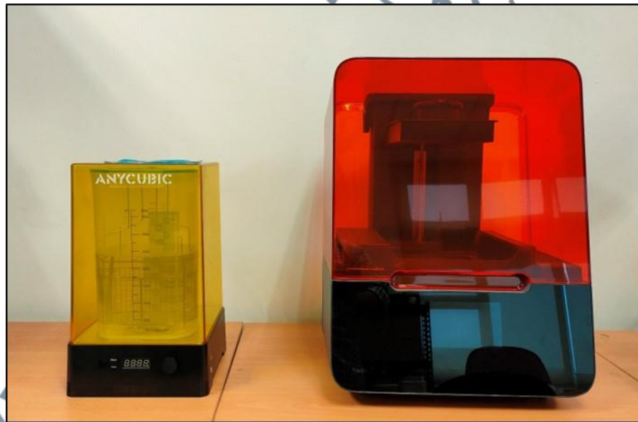
Figure 3.2: UV Cure Machine (Left) and SLA 3D Printer (Right).
