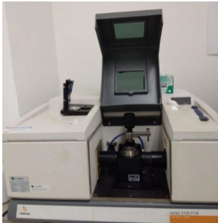
Figure 3.4: Varian 3100 Excalibur Series Fourier Transform Infra-Red (FTIR) Spectroscopy.
