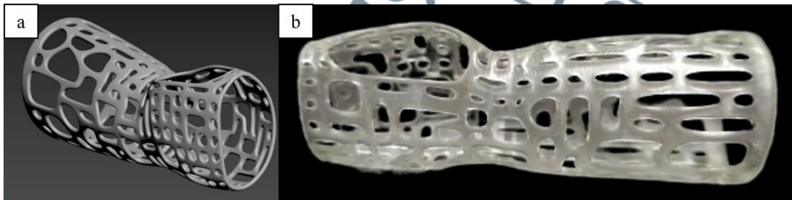
Figure 4.13: a) 3D Model Design; b) 3D Printed Arm Cast.
