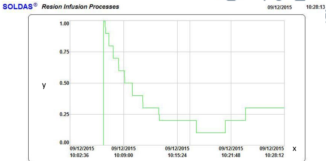
Figure 1: A sample of densified rosin-treated palm lumber, y: the pressure value and x: time during pressure.
