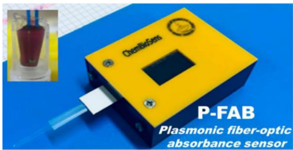
Fig. 10: P-FAB device and integrated U-bent fiber probe cartridge [11]
