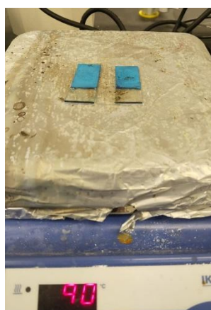
Fig. 3: Annealing process of the coated FTO glass at 90^\circ C .
