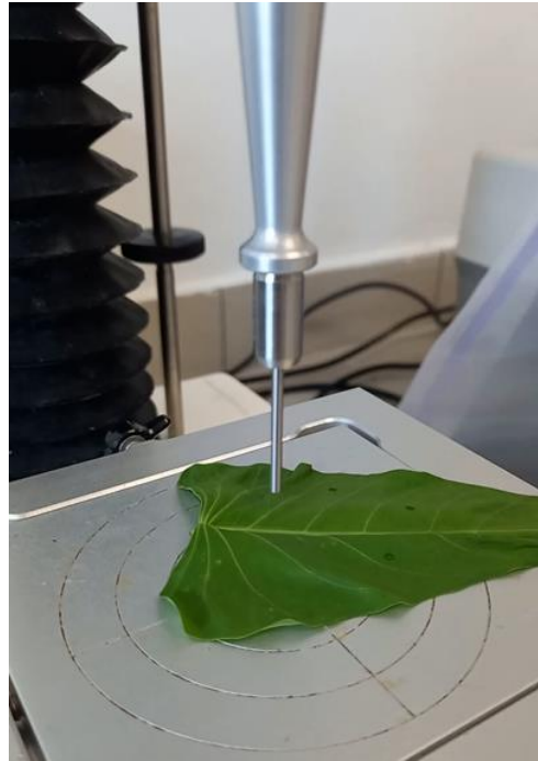
Figure 3.3: Set-Up for Leaf Firmness Measurement
