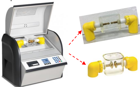
Fig. 2: AC breakdown tester (BAUR OIL -DTA 100C)
