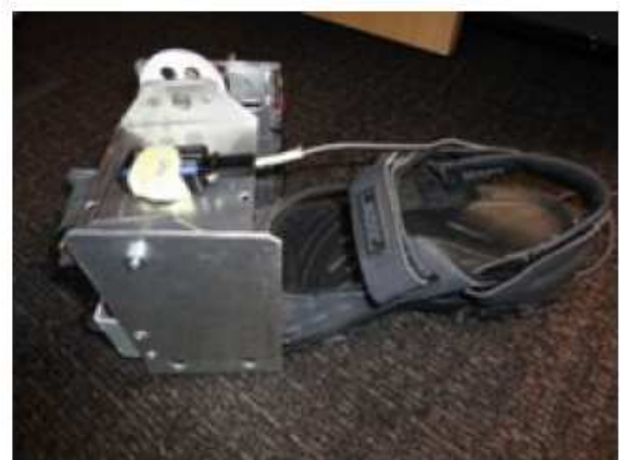
Fig. 1. RIMU prototype with IMU mounted on a rotating platform
