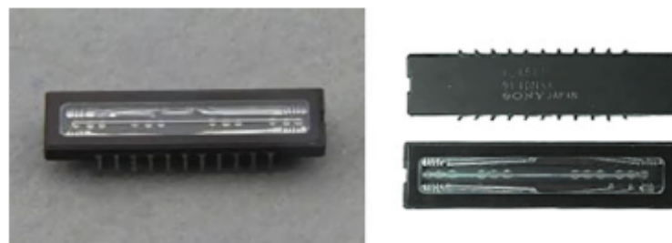
Fig. 1 CCD sensor ILX551A (left) [11] and ILX511 (right) [12]
