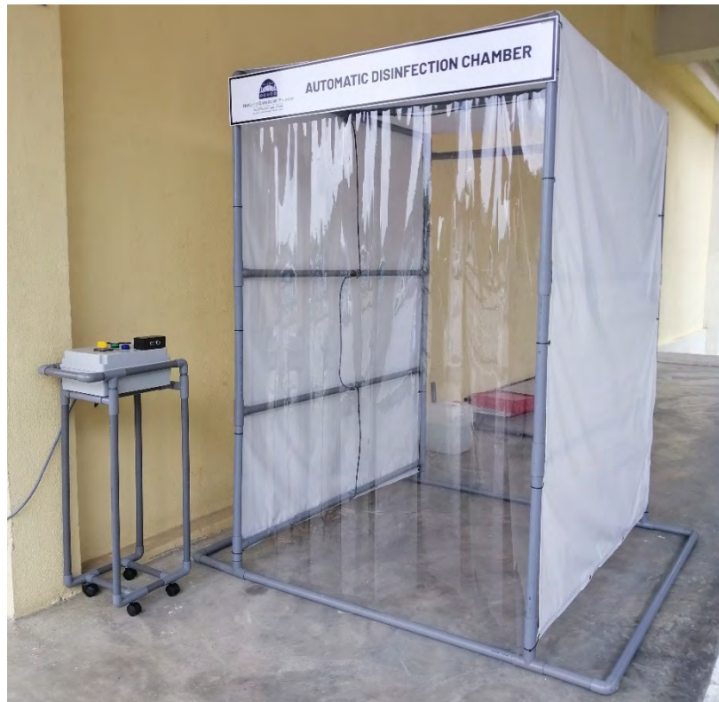
Figure 22 Fabricated low-cost automatic disinfection chamber.
