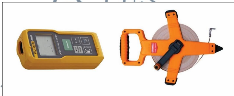
Figure 3.9: Laser Distance Meter Fluke 414D (left) and Kennedy 50 m/165 ft tape measurement (right)
