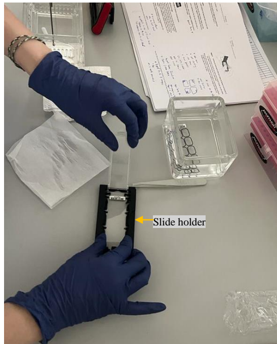
Figure 3.12: Placing the slide into the slide holder for scanning.
