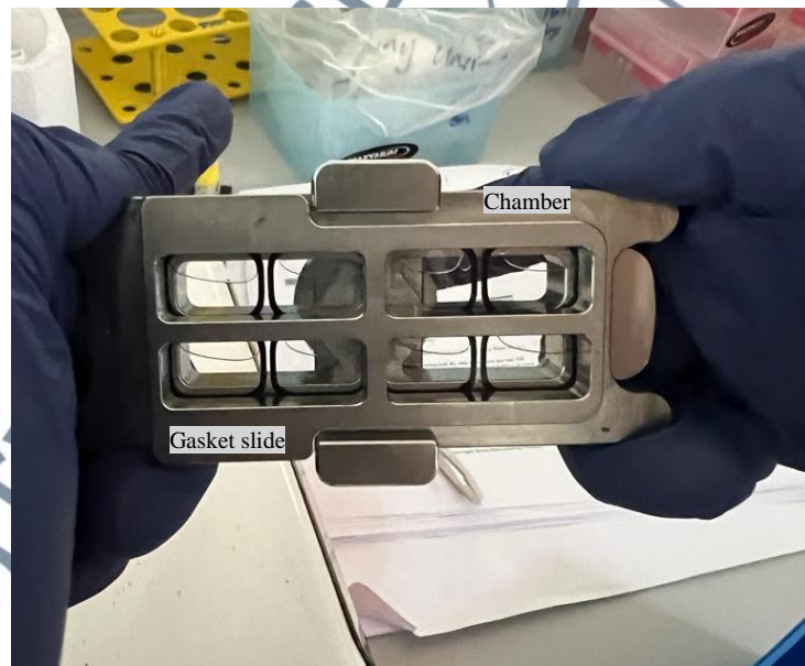
Figure 3.9: Assembling the chamber to the slide containing the sample.
