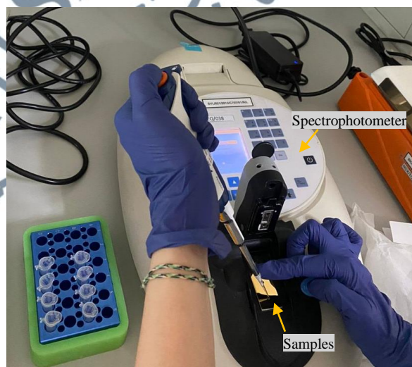
Figure 3.7: cRNA quality check using NanoDrop UV-VIS Spectrophotometer.
