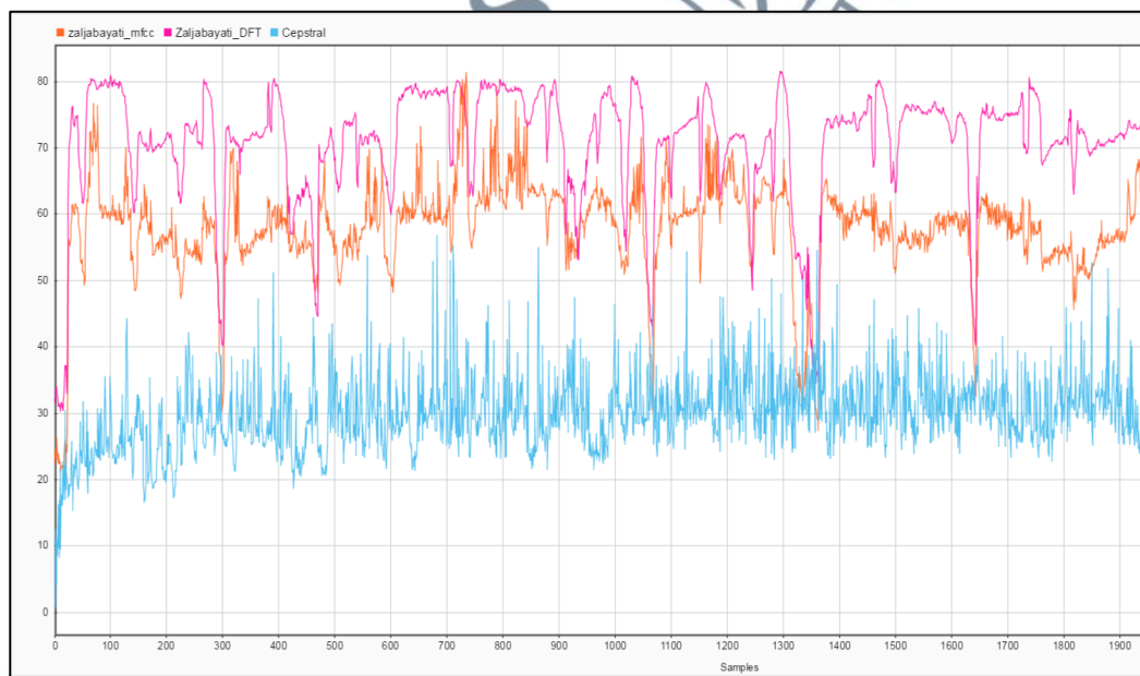
Figure 4.8 Sample of the overall performance for spectral envelope (formants) extracted using cepstral analysis (bottom graph), conventional MFCC (middle graph), and W-DFT (upper graph) for Maqamat Bayyati.
