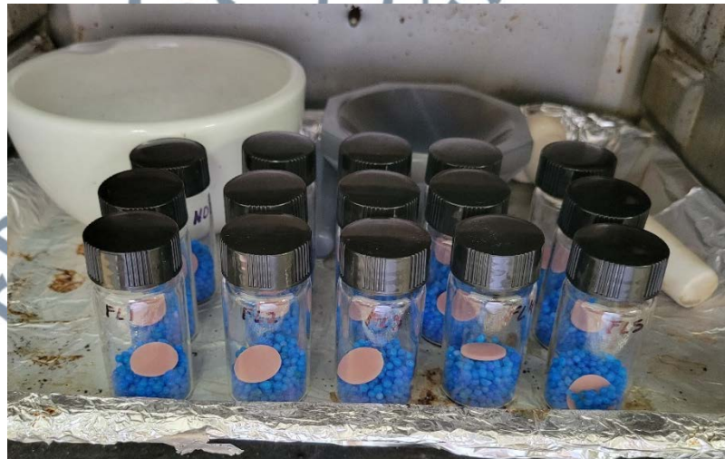
Figure 3.7: Specimens drying in independent desiccators in an oven at (37 \pm 1) ^\circ\text{C}
