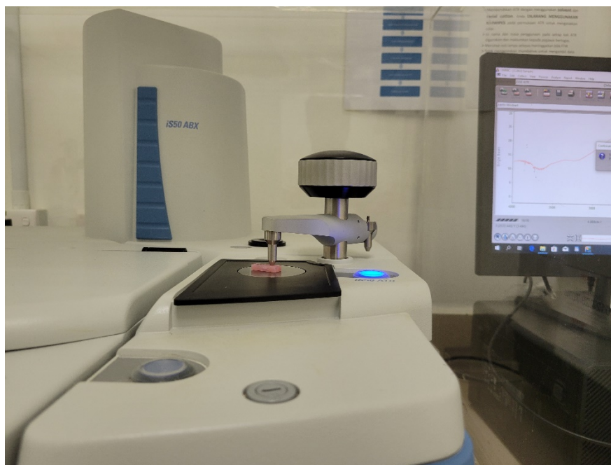
Figure 3.8: Examining the transmittance of the specimens using Fourier Transform Infrared (FTIR) spectroscopy
