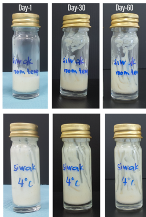
Figure 6: Physical appearance of Miswak gel stored at 4 °C and room temperature at day-1, day-30 and day-60.
