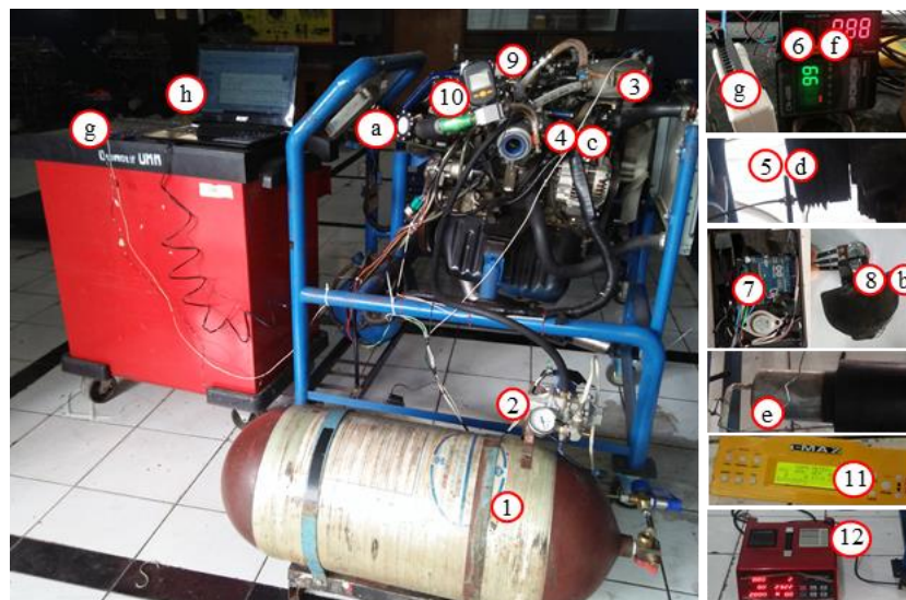
Figure 4. Data collection for the designed CNG control system
