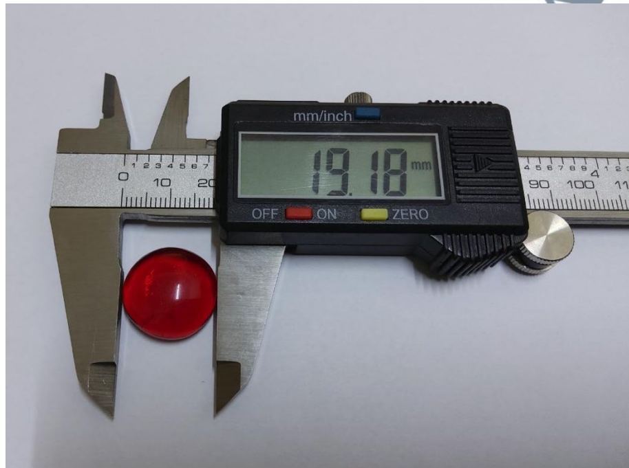
Figure 3.3: Diameter of Ruby Stone Z As Calculated Using a Vernier Calliper
